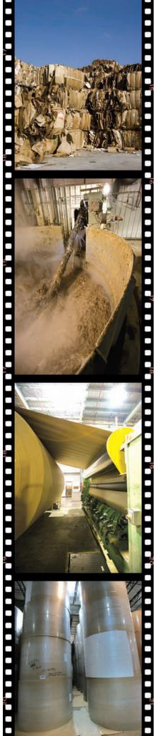
Pictured (top to bottom): Bales of recycled paper await transport to the stock prep area; bales enter the hydro pulper where they are pulped before being screened and cleaned; the sheet is transferred to the winder where it is cut to size; paper rolls are wrapped and labeled for shipment.
