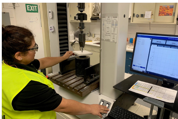
A Quality Lab Assistant at the Georgetown, South Carolina American Gypsum plant performs a nail pull test on a section of wallboard.
